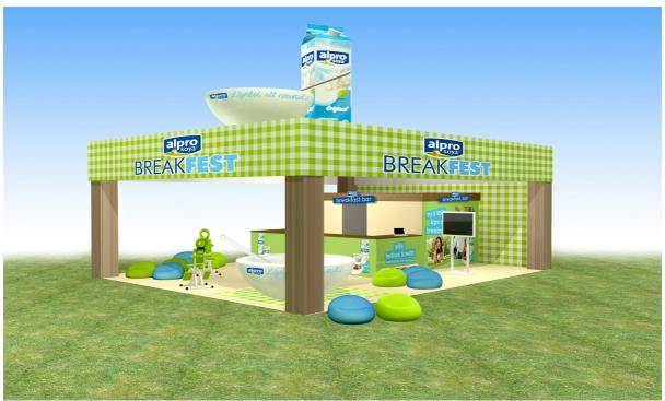
A 10mx8mx4m portal frame 'table' for promotional uses at a range of UK music festivals. Spaced legs of aluminium lattice truss provide frame rigidity under wind loading. The structure has since been modified to allow for increased loading from rigid carton, pot and bowl devices and an increase of 50% in the depth of the 'tablecloth' banner.
